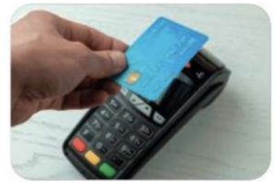
▲ Contactless card payments use RFID technology.
