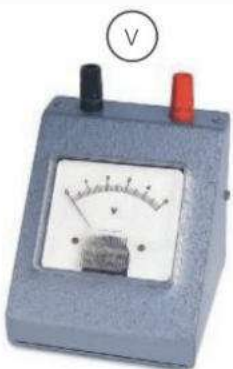
▲ Voltmeter and symbol. (For information about range and connection, see note under ammeter in previous spread.)
