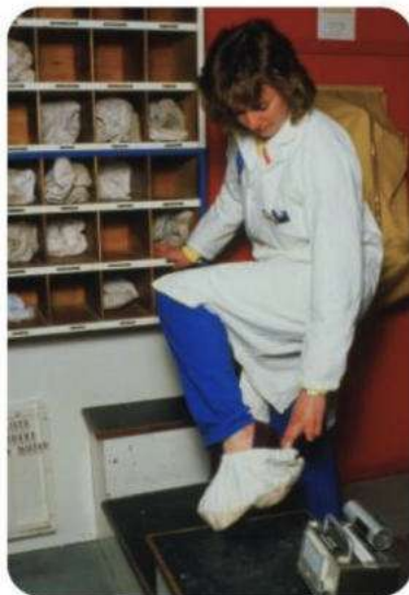
▲ This nuclear laboratory worker is about to use a GM tube and ratemeter to check for any traces of radioactive dust on her clothing
