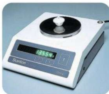
▲ The mass of an object can be found using a balance like this. The balance really detects the gravitational pull on the object on the pan, but the scale is marked to show the mass.
