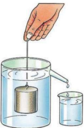
▲ Using a displacement can. Provided the can is filled to the spout at the start, the volume of water collected in the beaker is equal to the volume of the object lowered into the can.
