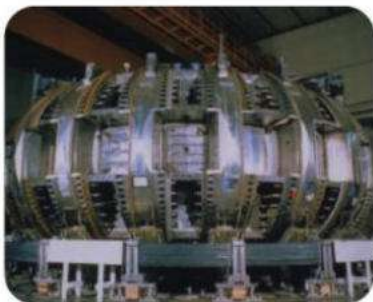
▲ This magnetic containment vessel, called a tokamak , is being used to investigate fusion
