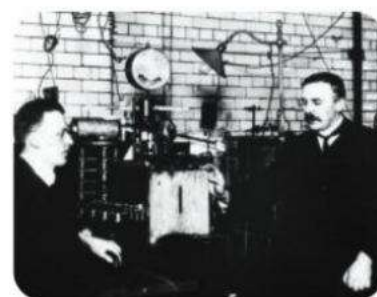
▲ Ernest Rutherford (right) and his assistant Hans Geiger, in 1912. They are standing next to the apparatus which they used for detecting alpha particles.
