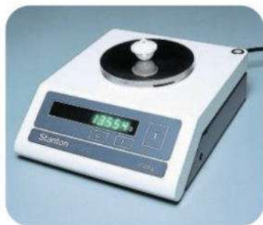
▲ A more modern type of balance. It detects the gravitational pull on the object on the pan, but gives its reading in units of mass.
