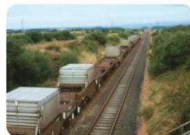
▲ The steel flasks on this train contain waste from a nuclear reactor
