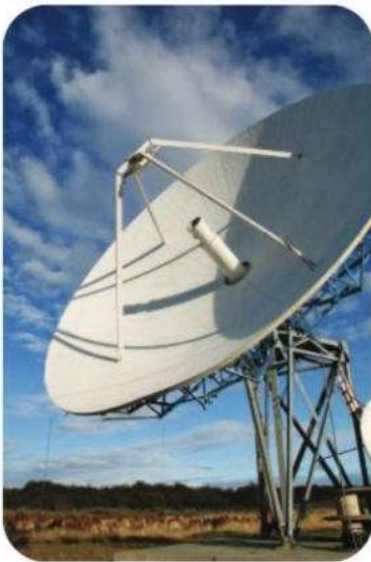
▲ This dish receives microwaves from a satellite.
