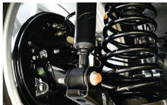
▲ Figure 17.12 Vehicle suspension system showing springs and dampers
