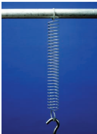
▲ Figure 5.6 The spring stores energy as it is stretched, releasing the energy as it returns to its original shape.
