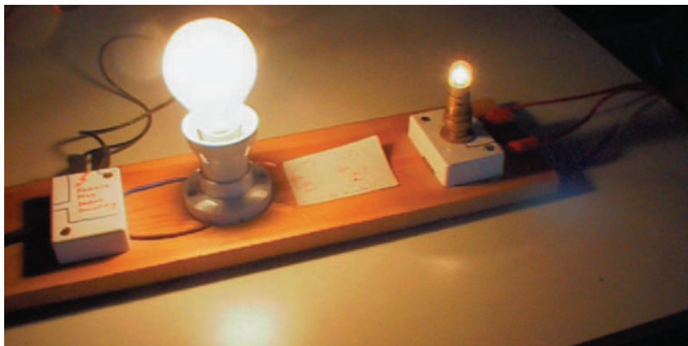
▲ Figure 9.4 A 240V, 100W mains lamp is much brighter than a 12V, 5W car light, but both have the same current. (Do not try this experiment yourself as it involves a large voltage.)
