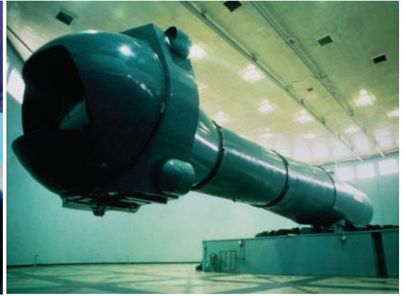
▲ Figure 12.10 Centrifuge testing the effect of acceleration on the human body
