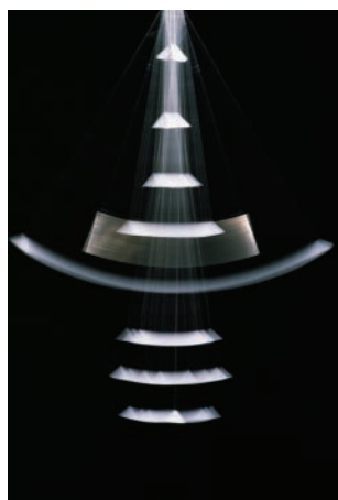
▲ Figure 17.17 Time-exposure photographs of Barton's pendulums with light damping, taken end-on. The longest arc, in the middle, is the driver.
