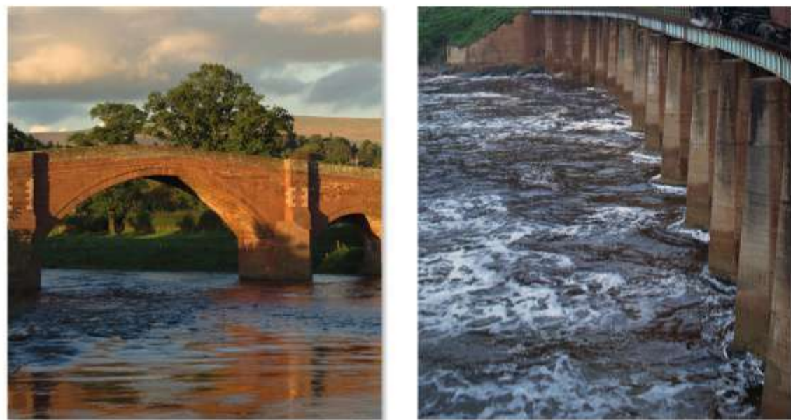
▲ fig D Increased speeds change streamline flow to turbulent flow.
