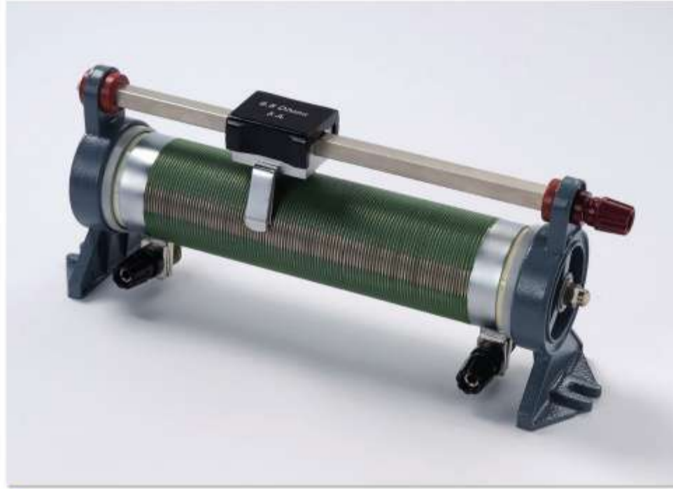
▲ fig E A potentiometer allows us to supply any voltage up to the maximum provided by our emf source.
