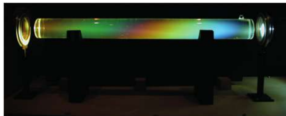
▲ fig G Sugar solutions can rotate the plane of polarisation. The degree of polarisation on a particular wavelength (colour) depends on the concentration of the solution, and how far the light has had to pass through it. This gives rise to the changing colours seen along the length of this tube of sugar solution.
