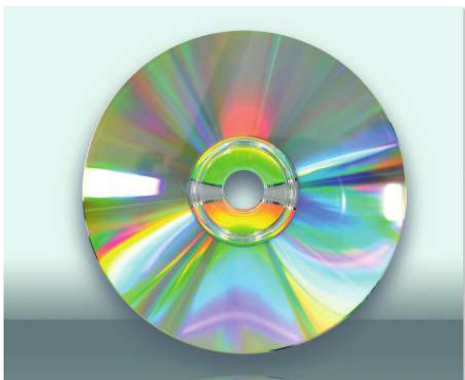
▲ fig H CDs have a series of very close lines marked on them and act as a diffraction grating that reflects. This causes the spectrum of colours that can be seen on them from white light that hits the surface.
