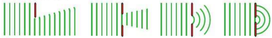
▲ fig D The amount of diffraction depends on the size of the gap relative to the wavelength.
