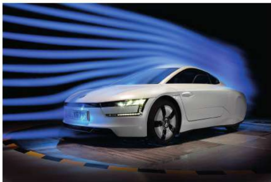
▲ fig C Smoke streamlines show laminar flow of air over a well-designed car.
