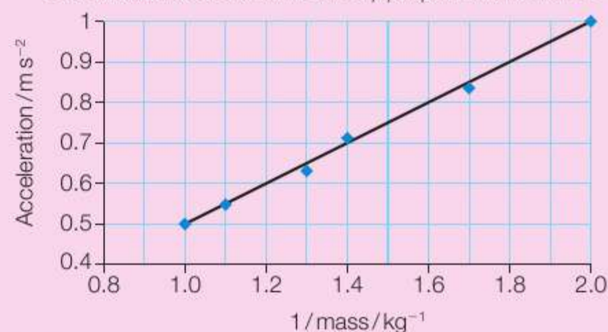
fig E Graph of results from the second investigation into Newton's second law. The x-axis represents the derived data of '1/mass', so the straight best-fit line shows that acceleration is inversely proportional to mass. Note that there is no need for a graph to start at the origin: choose axes scales that will best show the pattern in the data by making the points fill the graph paper.
