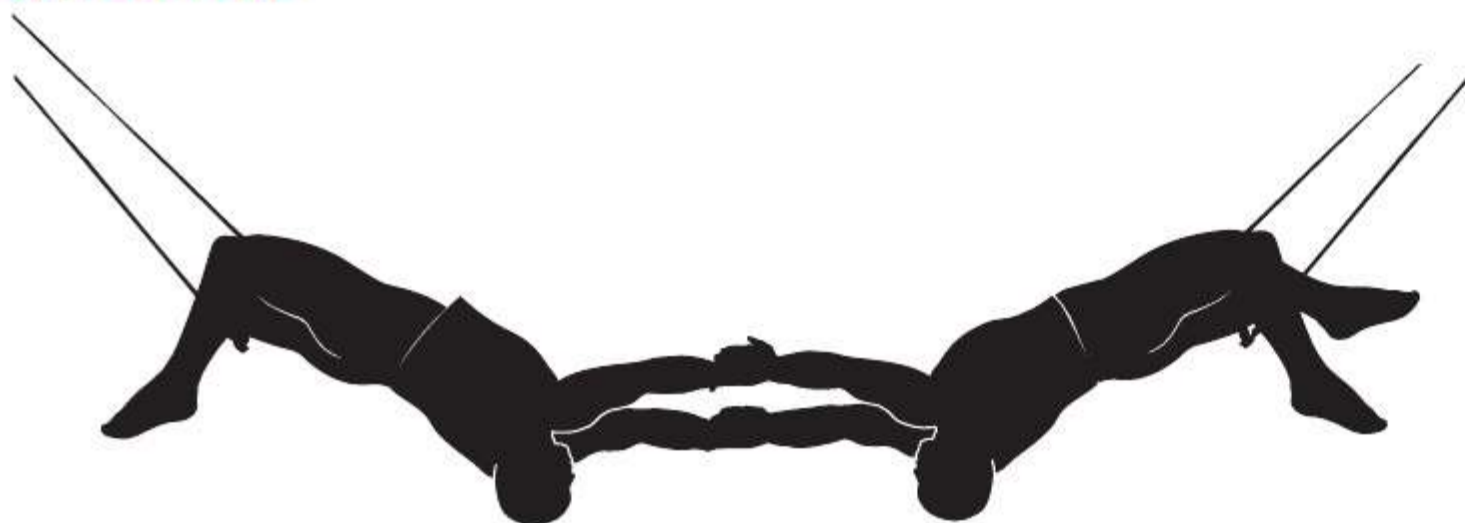
▲ fig C In this illustration, these trapeze artists are stationary. If they let go of each other, they will 'explode' – they will fly apart with equal and opposite momenta.
