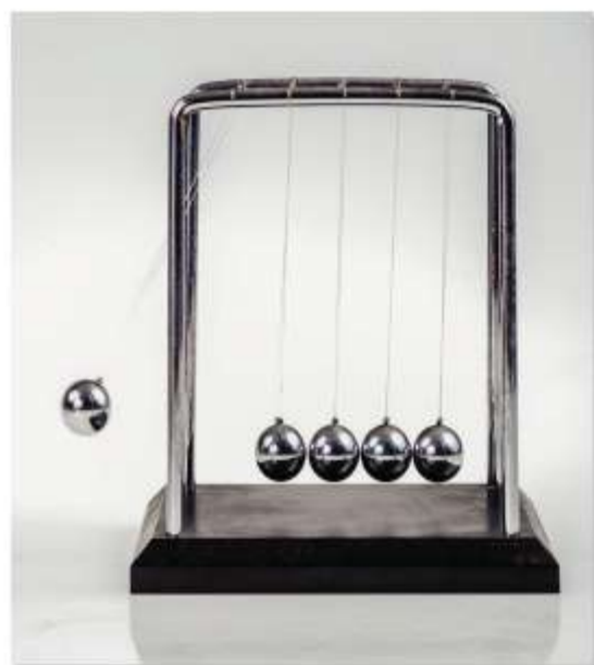
▲ fig A Newton's cradle: each time the balls collide, momentum is transferred from one to another, but the total momentum remains constant.
