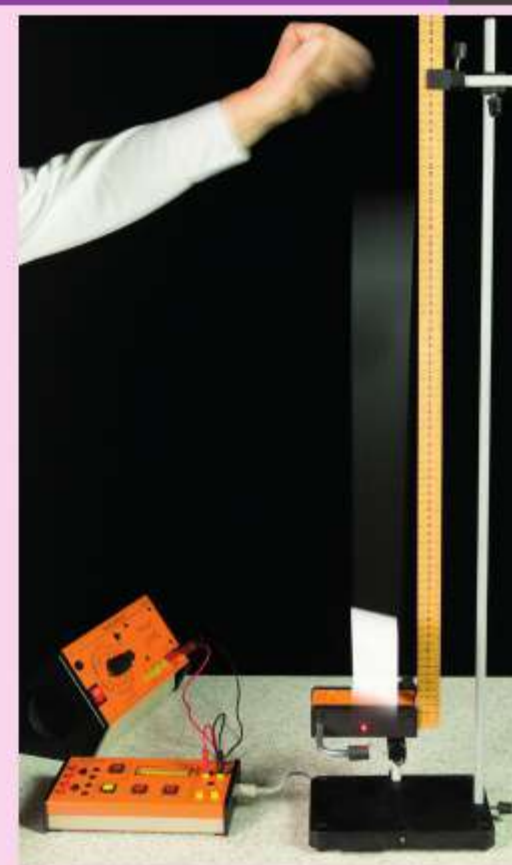
fig E The freefall velocity of an object from different heights allows us to find the gravitational field strength, g .
