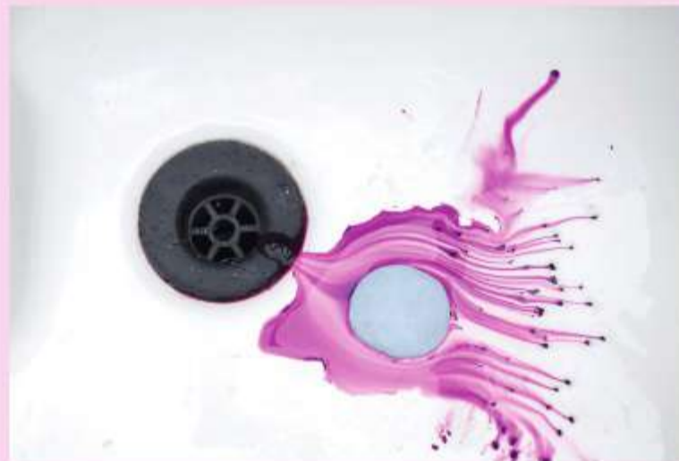
▲ fig E A few crystals of potassium manganate(VII) will produce purple trails in the water flow which can then be made to pass around objects made from clay. You can alter the flow rate and the obstacle shapes in order to see how the flow changes.
