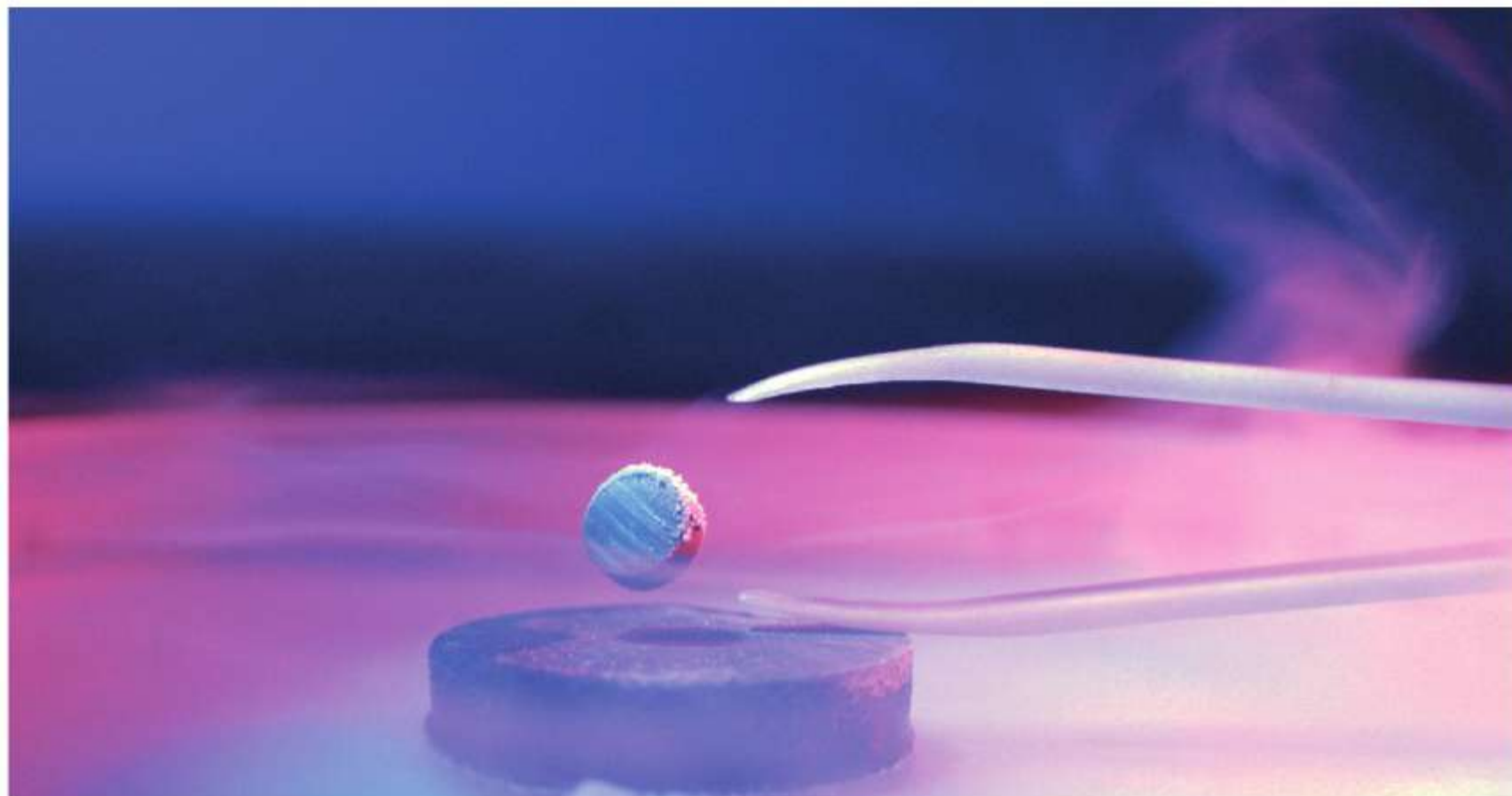
▲ fig D Superconductors can levitate magnets, as they do not accept penetration by magnetic fields. This is the Meissner Effect.
