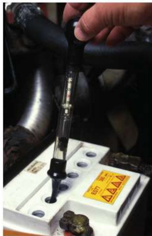
fig D A hydrometer can check the density of battery fluids, which tells us if the fluids need changing.
