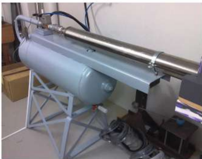
▲ fig C Ball cannon capable of speeds in excess of 200 km h.
