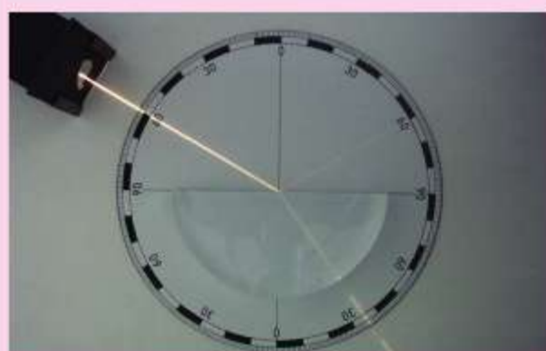
fig D Measuring angles of incidence and refraction in order to find the refractive index of a material.
