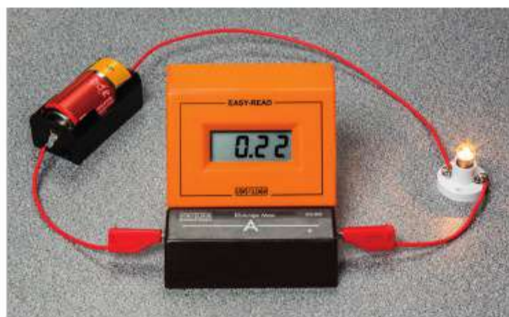
▲ fig B We can measure electric current through a component using an ammeter connected in series.
