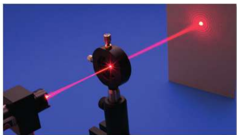
▲ fig A Circular diffraction pattern caused by a laser passing through a pinhole.
