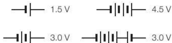
▲ fig E Emfs in series will add up. Take care to account for their direction, as cells in opposite directions oppose each other and cancel out the emf they would supply.
