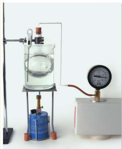
▲ fig D Apparatus to demonstrate the pressure law. The temperature and pressure readings could be taken by electronic sensors and the data logged by an attached computer.
