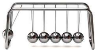
▲ fig B Newton's cradle maintains kinetic energy, as well as conserving momentum in its collisions.
