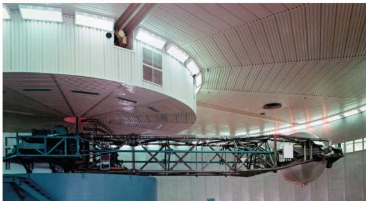
▲ fig B Astronauts are subject to extreme acceleration forces. These forces are simulated in training by the centripetal force in a giant centrifuge.
