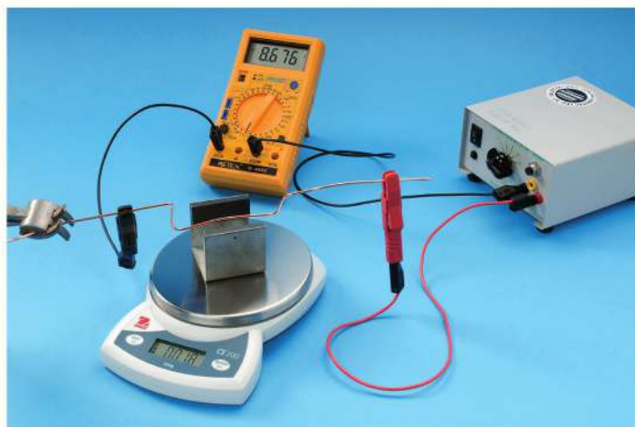
fig A Investigating the strength of the force on a current-carrying conductor in a magnetic field.
