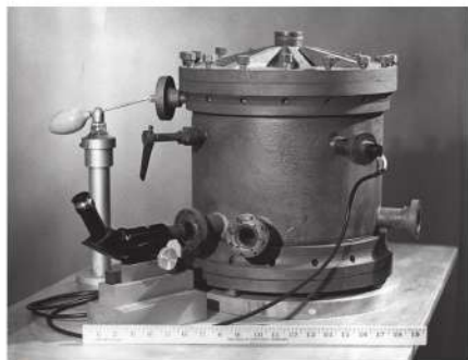
▲ fig F Millikan's oil drop apparatus for finding the charge on an electron. The chamber shown was suspended in a trough of motor oil to reduce heat transfer within it, and so reduce any problems of convection currents affecting falling oil droplets within the chamber.
