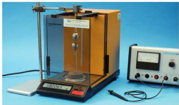
▲ fig B Measuring the force between two charges.
