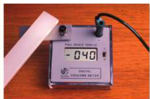
▲ fig C A coulombmeter will measure how much charge is stored.
