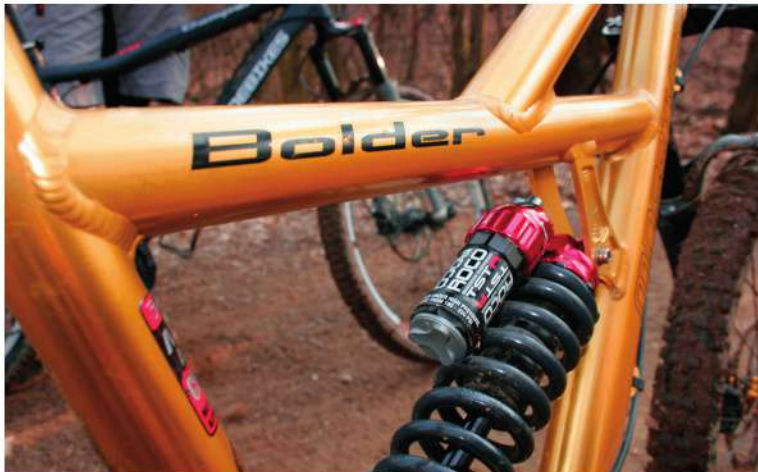
▲ fig H Mountain bike suspension has springs to accept some movement, and shock absorbers to critically dampen any oscillations.
