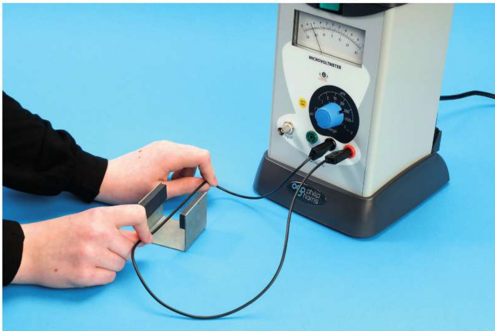
▲ fig A Relative movement between a wire and a magnetic field will induce an e.m.f.
