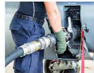
▲ Figure 9.17 Earthing during refuelling
