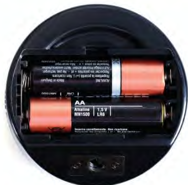
▲ Figure 7.7 When one coulomb of charge passes through both these cells in turn it gains 3 J of energy.
