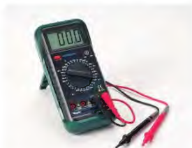
▲ Figure 7.3 An ammeter is used to measure current in a circuit. It has a very low resistance and so has almost no effect on the current.
