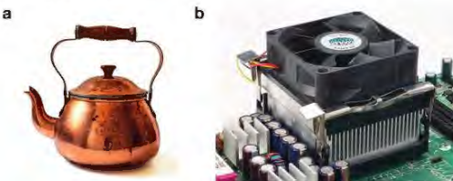
▲ Figure 15.13 a A shiny kettle stays warmer longer. b The heat sink needs to be matt black to lose heat to the surroundings quickly, and so stop the transistor overheating.
