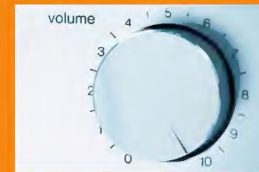
▲ Figure 8.1 Turning this dial alters the resistance in the circuit which changes the volume of the sound.
