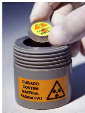
▲ Figure 24.9 Radioactive samples are stored in lead-lined containers and are handled with tongs or protected fingers.
