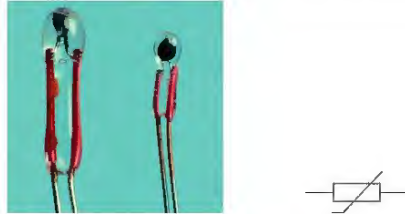
▲ Figure 8.14 Two examples of thermistors and their symbol – the resistance of a thermistor changes a lot as the temperature changes.
