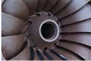
▲ Figure 17.10 The turbine has angled blades. As water is forced between the blades, they start to turn. The rotating turbine is connected to a generator to make it turn too.
