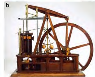
▲ Figure 16.10 a James Watt (1736–1819) was a Scottish engineer who improved the performance of the steam engine and can be said to have started the Industrial Revolution – the beginning of the machine age. b A model of a steam engine that transfers the heat energy of steam to movement. Watt's engines were used to pump water out of mines.
