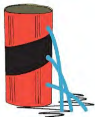
▲ Figure 18.9 Pressure in a liquid increases with depth.
