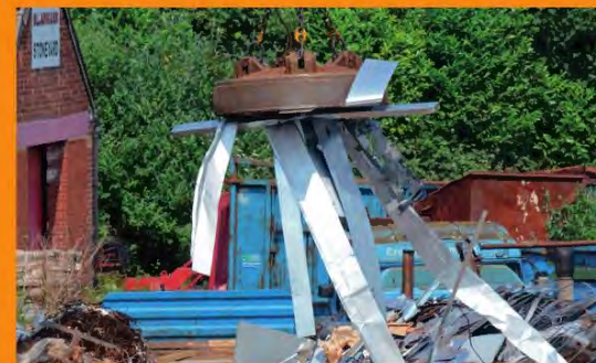
▲ Figure 20.1 Electromagnets can be used to lift iron or steel objects.
