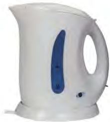
▲ Figure 6.8 This plastic kettle has double insulation which means that there is no need for an earth wire.
