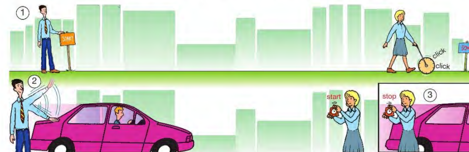
▲ Figure 1.4 How to measure the speed of cars driving on the road
