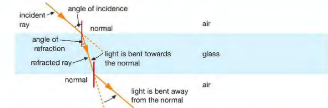
▲ Figure 12.7 This light ray is being refracted twice – once as it travels from air into glass and then as it travels from glass to air.
