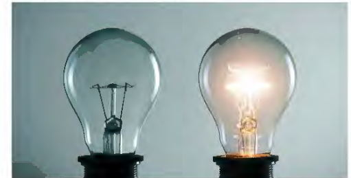
▲ Figure 6.11 It is the heating effect of a current that is causing this bulb to glow.
