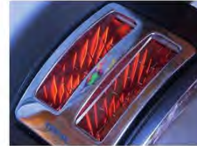
▲ Figure 6.10 The wires inside a toaster have a high resistance. They become very hot when a current passes through them.
