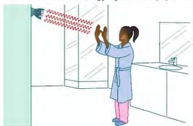
▲ Figure 15.9 Heat is transferred from a heater by radiation.
