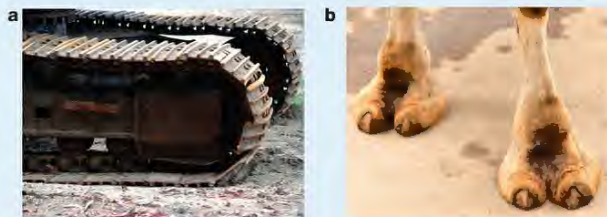
▲ Figure 18.5 a The caterpillar tracks on this vehicle spread its weight over a large area. b Camels have large feet so they are less likely to sink into loose sand.
