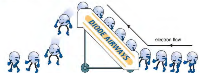
▲ Figure 8.17 Diodes will only let charges flow one way.
