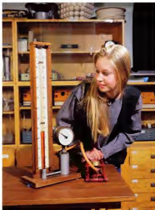
▲ Figure 19.8 A modern version of Boyle's experiment to see how the volume of a gas depends on the pressure exerted on it.
