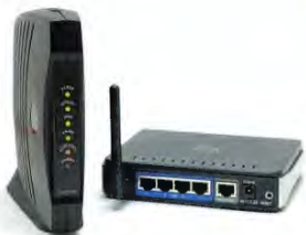
▲ Figure 7.11 Glowing LEDs indicate which circuits are working
