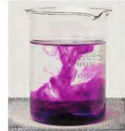
▲ Figure 15.4 Demonstration of convection currents, using a potassium manganate (VII) crystal in water
