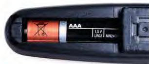
▲ Figure 7.6 When one coulomb of charge passes through this cell it gains 1.5 J of energy.
