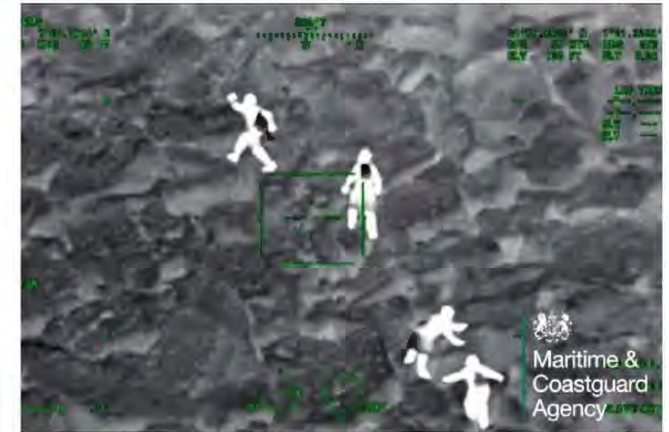
▲ Figure 11.5 It is not possible to see these people trapped at the bottom of a cliff using normal visible light. By using infrared detectors they can be found easily and rescued.
