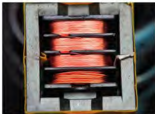
▲ Figure 21.15 A transformer
